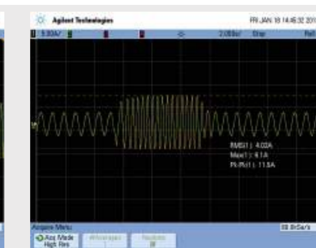
Current waveform in sudden acceleration/deceleration at 0.5Hz
