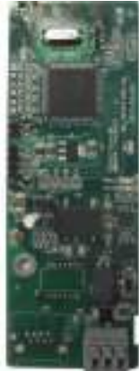
CANopen/CAN master/slave control communication card EC-TX505/511
