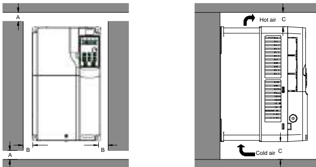
Figure 4-3 Installing one VFD
