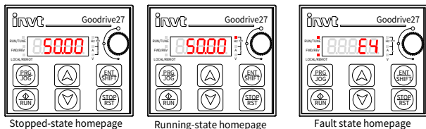
Figure 5-2 Status interface display
